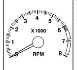
The tachometer displays the engine speed in revolutions per minute (rpm).
